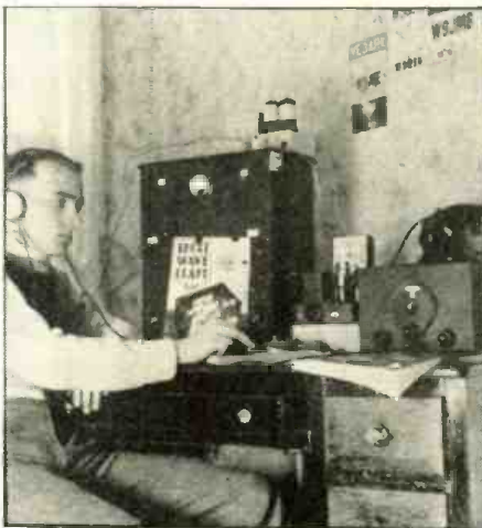
The photo above shows the Ham station of Joseph Horvath, W8QKA, 3710 Wellington Ave., Parma, Ohio. Receiver used is a National AC-58 and the power supply unit is home-built. The transmitter at the left of the desk is a 6L6M crystal tritret with a 10 final amplifier. The frequencies used are 3633 and 7266 kc.
