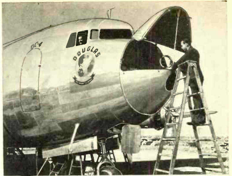
E. A. Post, communications engineer of United Air Lines, inspects the DC-4's direction-finding loop antenna. Two additional receiving antennas are installed beneath the ship and a transmitting antenna above her.
